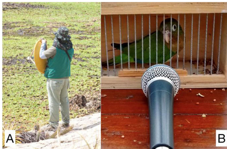
Fig. 2. Recording setups used for Cactus Conure ( Eupsittula cactorum ) sound recordings. Recordings of wild individuals were made using a parabolic dish (A); captive individuals were recorded at close range with the same cardioid microphone (B).
